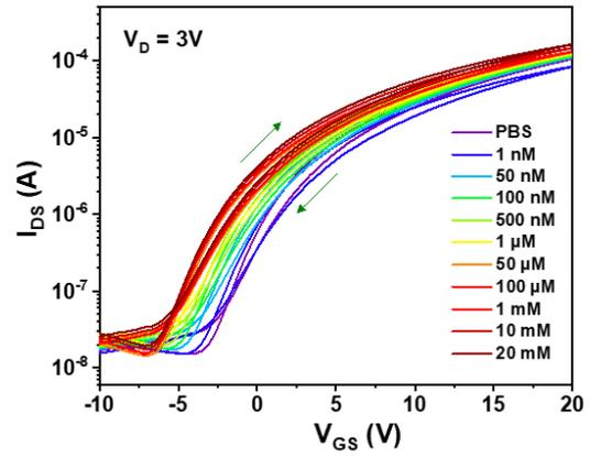
Fig. 2. Transfer characteristics of Bio-FET for glucose concentrations (1 nM to 20 mM) in 0.1x PBS.
