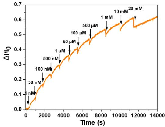
Fig. 3. Real time measurement current changes as a function of time with glucose concentration (1 nM to 20 mM) in 0.1x PBS.
