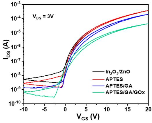
Fig. 1. Transfer characteristics of Bio-FET of bare, after APTES, GA and GOx enzyme functionalization.
