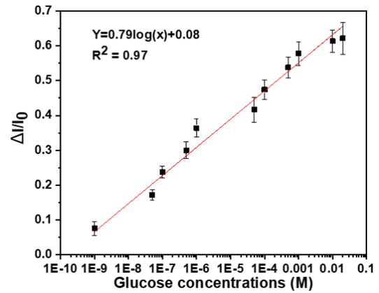
Fig. 4. Calibration plot of Bio-FET based on the real time measurement, Error bars denoted mean the average and standard deviation values (mean  $\pm$  SD) for three independent measurements (n=3).
