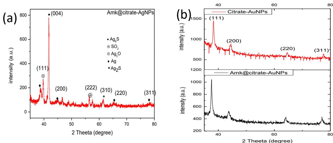
**Fig.1.** XRD pattern for (a) Amk@citrate-AgNPs and (b) citrate-AuNPs and Amk@citrate-AuNPs,
